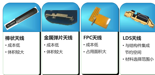
Figure 5-7 Recommended Types of Conventional Antennas for NB-IoT
