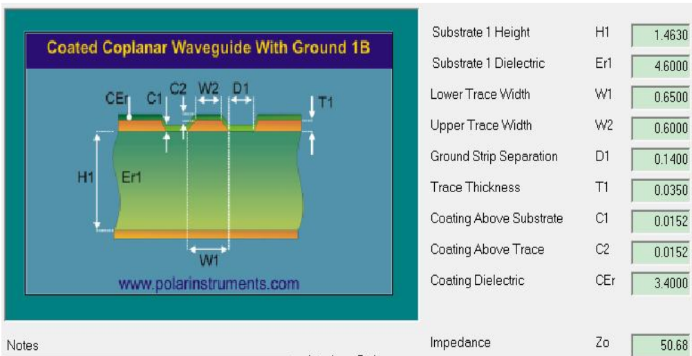
Reference for the calculation method of 50\Omega impedance in Figure 5-5
